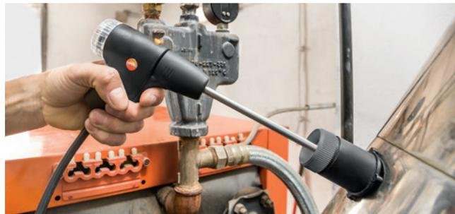
Thanks to the testoFix probe mount, the flue gas probe is always securely positioned in the core flow.
