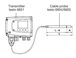
L = Probe length L-A = Probe length – length protective cal A = 35 mm
