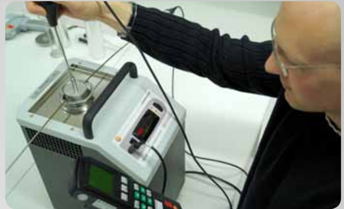
surface insert with external working standard, control sensor and test specimen
