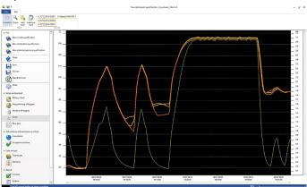
Tools like axes configuration, formula and curves are available for analyzing the measurement curves:
