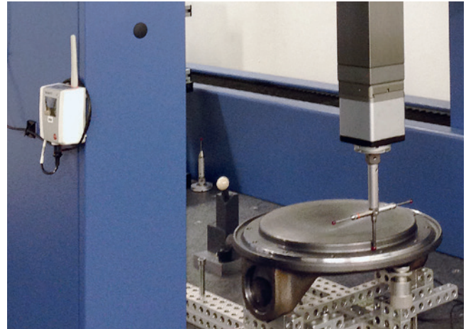
Monitoring ambient conditions in a measurement room with a testo Saveris data logger.
