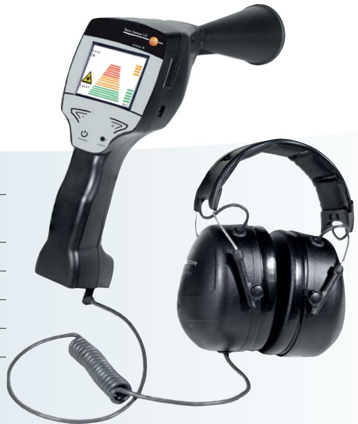
Gases escaping from leaks in pipe systems (e.g. corrosion, untight screw connections etc.) cause noises in the ultrasonic range. With the testo Sensor LD, even the smallest leaks, which are not audible for the human ear, and due to their size are not visible, can already be localized from several metres away. The testo Sensor LD converts the inaudible ultrasound into audible frequencies. These sounds can be perceived even in loud surroundings with the comfortably worn, sound-proof headphones.
