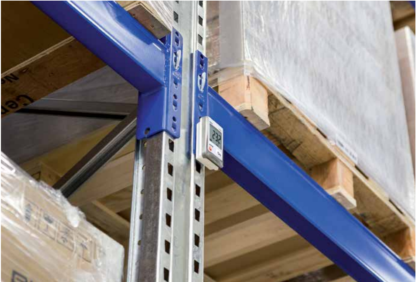
Any limit value violations can still be identified easily in the large display of the data logger, even if it is installed at a greater height.
