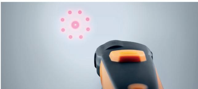
A red laser automatically marks the measurement spot of the infrared thermometer testo 805i. This lets you see exactly what you are measuring – and what not. By the way: you also see this mark in the report you create with the testo Smart Probes App.
