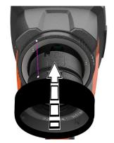
2 Align the markings on the lens and handle.
