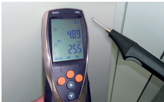
Humidity measurement on sensitive goods without opening cabinet doors.
