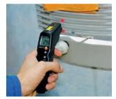
testo 830 measures the surface temperatures of walls, ceilings and floors using infrared technology. This allows points which are too cold, at which humidity could precipitate, to be determined and if necessary countermeasures taken.
