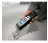
testo 616 measures material moisture non-intrusively using a contact probe in wood, screed, cement and concrete at a depth of up to 5 cm. The instrument simplifies the work of anyone who must observe the drying processes of floors, walls and surfaces as well as moisture damage.
