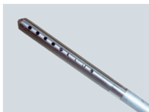
Thin measuring tip with a 4 mm diameter.
