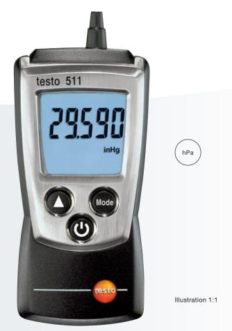
testo 511 measures absolute pressure to an accuracy of  $\pm 3$  hPa. The measuring instrument is ideal for absolute pressure compensation during flow velocity measurements with a Pitot tube, for example. By entering the altitude above sea level, this is converted into barometric air pressure. In addition to this, a barometric pressure measurement between two points is also possible. The eight switchable pressure units offer the user highest flexibility in measurement.
