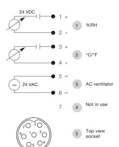
DC: Supply transmitter AC: Supply ventilator
