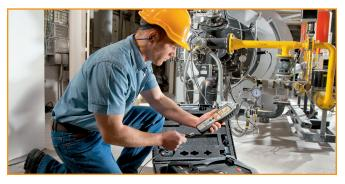
Industrial boilers and burners have their own unique characteristics. When an unexpectedly high CO is detected, **the testo 350 will automatically adjust to the situation,** keeping the sensor protected at all times.
