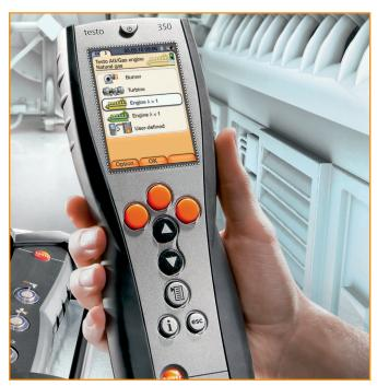
Use the control unit of the testo 350 remotely from a comfortable location up to 300 feet away (with Bluetooth), instead of up on the stack.
