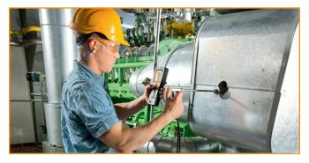
Rich-burn engine exhaust, when uncontrolled, can have wide concentration ranges and both CO and  $NO_x$  can fluctuate significantly. The on-board CO dilution system will automatically set-up for optimum testing, perfect for a rich burn engine. Lean-burn engines have different exhaust characteristics, but  $NO_2$ can make up a significant portion of the total  $NO_x$  measurement. The 350 measures both NO and  $NO_2$  for proper lean-burn engine set-up.
