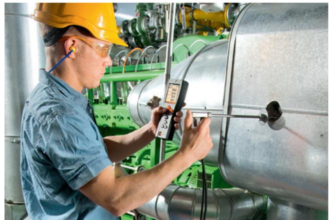
Fig. 2: testo 350 exhaust gas measurement at the engine
