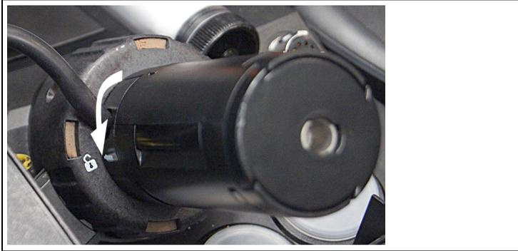
2. Unlock the preheating section (anti-clockwise) and remove.
