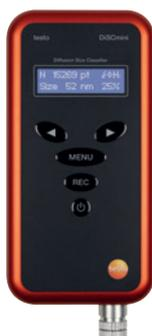
The nanoparticle measuring instrument
