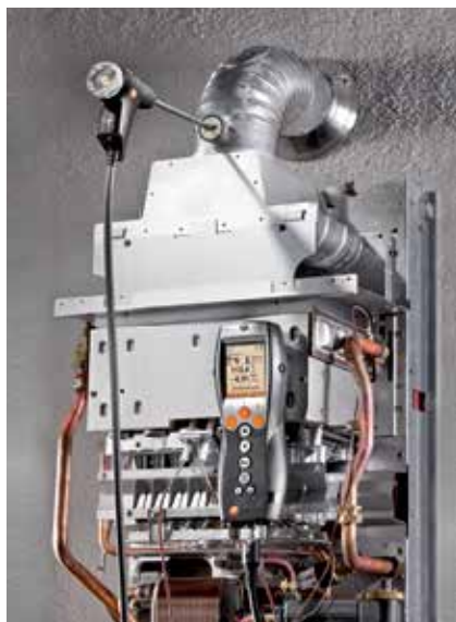
Fig. 8: A flue gas analyzer, e.g. testo 330, is essential for carrying out adjustments
