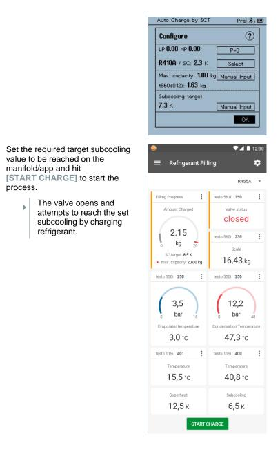
Added refrigerant is displayed in g/kg increments on the manifold/app.
