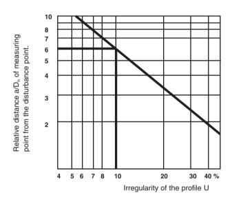
The uncertainty of the measurement location is obtained from the accepted number of measuring points = 10:  $T_U$  =7 %.
