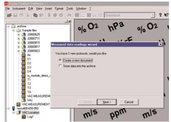
Connect the instrument to the PC. After starting Comsoft and selecting testo 400, the current memory contents are displayed. Select the required protocol and the lcoation and then drag the file to the work area by keeping the right mouse button pressed. Select the "Form" Inview type from the toolbar.
