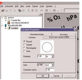
Select the location beforehand and enter the duct cross-section (round or rectangular for use by the VAC module). For "Correction factor" it is possible to enter a value which will correct the area and consequently the calculated volume flow in relation to the measuring location. For example:
