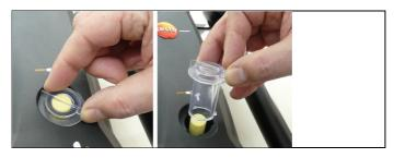
Open the filter chamber: Turn the filter cover anti-clockwise and take it off.
