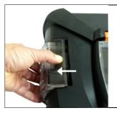
2. Unlock the condensate trap / condensate container and pull it vertically off the meas. box.
