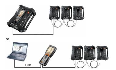
If testo easyEmission software is connected via a control unit to measuring boxes, the number of measuring boxes must not be changed. To add new measuring boxes, end the testo easyEmission software, connect the new measuring box and restart the testo easyEmission software.
