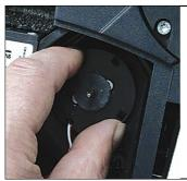
4. Loosen the motor on the condensate pump (short anticlockwise turn).
