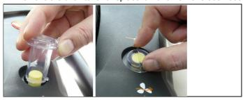
3. Attach the filter cover and lock by turning it clockwise. The rib on the filter cover must be parallel to the handle.
