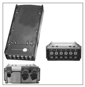
The analog output unit 0554 3149 (accessory) is suitable for the output of up to 6 measuring channels in the form of analog signals (4 to 20mA). The analog output unit is connected to the instrument via data bus, and the configuration can be carried out via the control unit.
