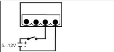
Occupying the trigger input, with supply via instrument voltage (12 V):
