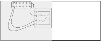
In both channels the positive output is connected to the ground connection of the recorder. The interfaces work correctly.
