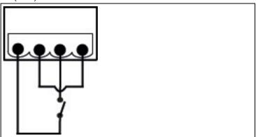
In case of supply via instrument voltage the flue gas analyser can only be started via the trigger input from switched off state when the mains plug is plugged in.
