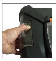
1. Unlock the condensate trap / condensate container by the orange handle on the underside.
