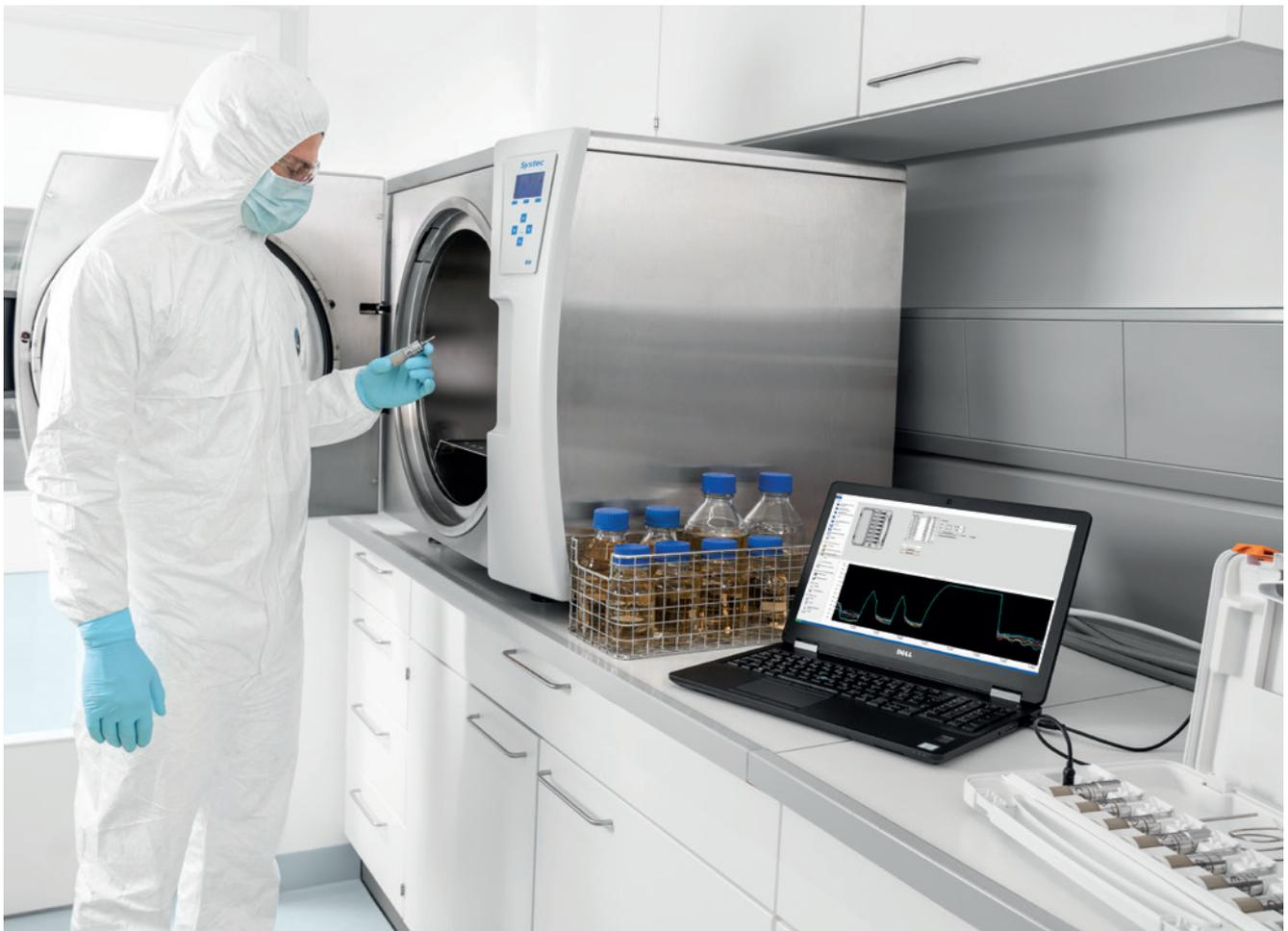
In order to ensure security in the manufacture of medicaments in autoclaves, the sterilization of pharmaceutical products has to meet high GxP requirements and be CFR 21 Part 11-compliant. These critical processes must be validated at regular intervals. For this purpose, cabled and wireless systems are today in use for measuring temperature and pressure. When using these systems, Excel lists with complex calculations are frequently used as standard-compliant documentation.
