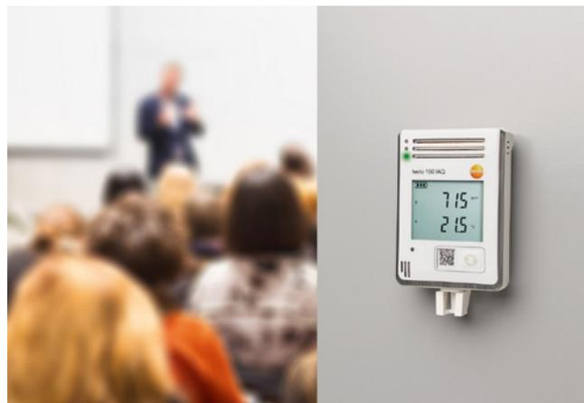
The testo 160 IAQ WLAN data logger in use.
