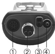
① **Probe socket:** Connect probes before the measuring instrument is switched on, or switch the instrument off and then on again after a change of probe.
