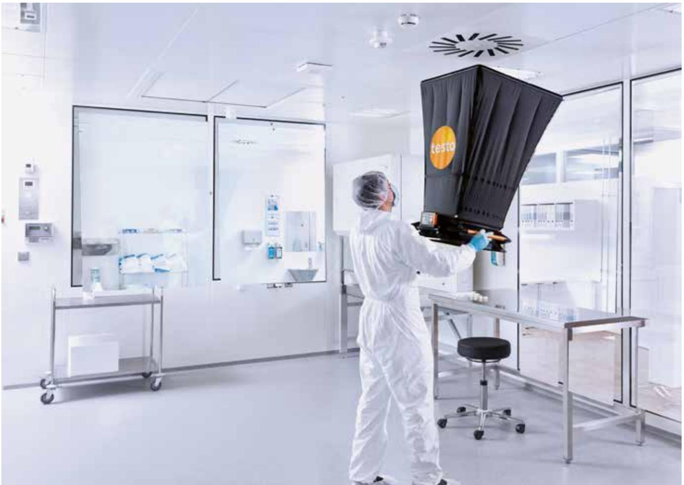
VAC systems in cleanrooms must meet strict legal hygiene requirements. In order for the various norms and guidelines for these standards to be adhered to, the prescribed air exchange rate of a room must be regularly ensured by testing the total volume flow of the system. These checks are often carried out at larger swirl outlets which distribute the air evenly. The problem at swirl outlets: the turbulent air can severely falsify the measurement result. With the volume
