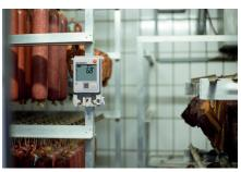
Refrigerated room monitoring at the butcher's (testo Saveris 2-T2 with external NTC probe with door contact)
