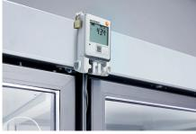
Ultra low-temperature freezer monitoring in laboratories (testo Saveris 2-T3 with temperature probe)
